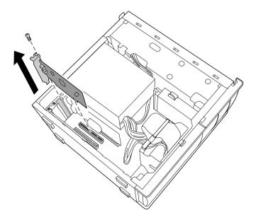
Grasp the card with one hand on each end, and gently pull up as you rock the card from side to side. Hold the add-in card by its edges and do not touch any components or contacts on the card. Static electricity in your body may damage sensitive components on the card. As a precaution, touch any exposed metal part on the metal chassis (preferably the metal part on the power supply) before handling an add-in card to discharge any static electricity in your body.
